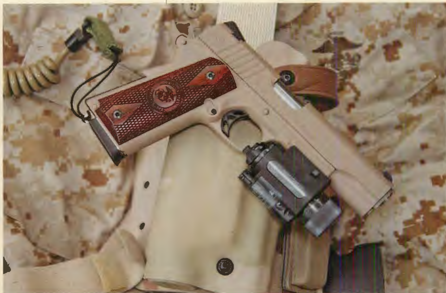
Para-Ordnance's USMC pistol is a single-action finished in Coyote Brown. It is seen here with Safariland's 6004 Series USMC LightMount holster with an Insight M3 Tactical Light mounted on its M1913 frame rail.
